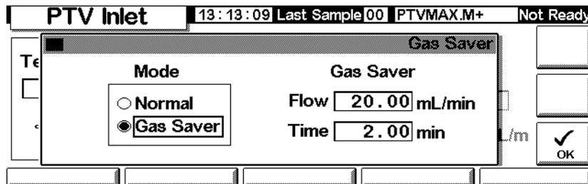
7. Press Prep Run before manually injecting the sample if the Gas Saver is on (see page 68).
