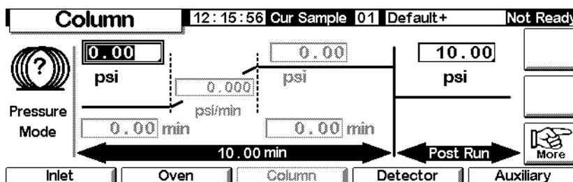
2. Note the question mark at the left, indicating that the column is not defined. To define it, press More, select Configure Column, and press Enter to display the next screen.
