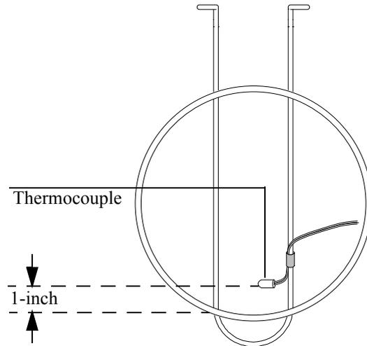
**Figure 24. Thermocouple and column hanger**
