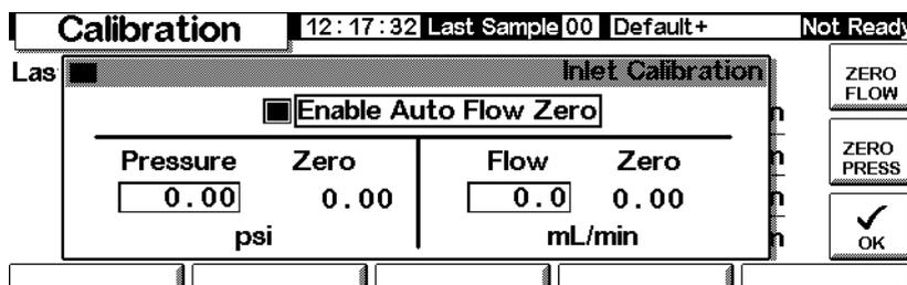
2. Select Enable Auto Flow Zero to automatically recalibrate the zero at the end of every run.
