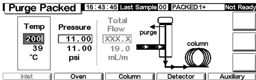
2. Set the inlet temperature and pressure for the method.
