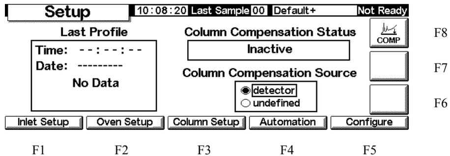
3. Press Column Setup to get to the next screen. The second version shown below appears with Auxiliary EPC GCs. The first screen appears with all others.
