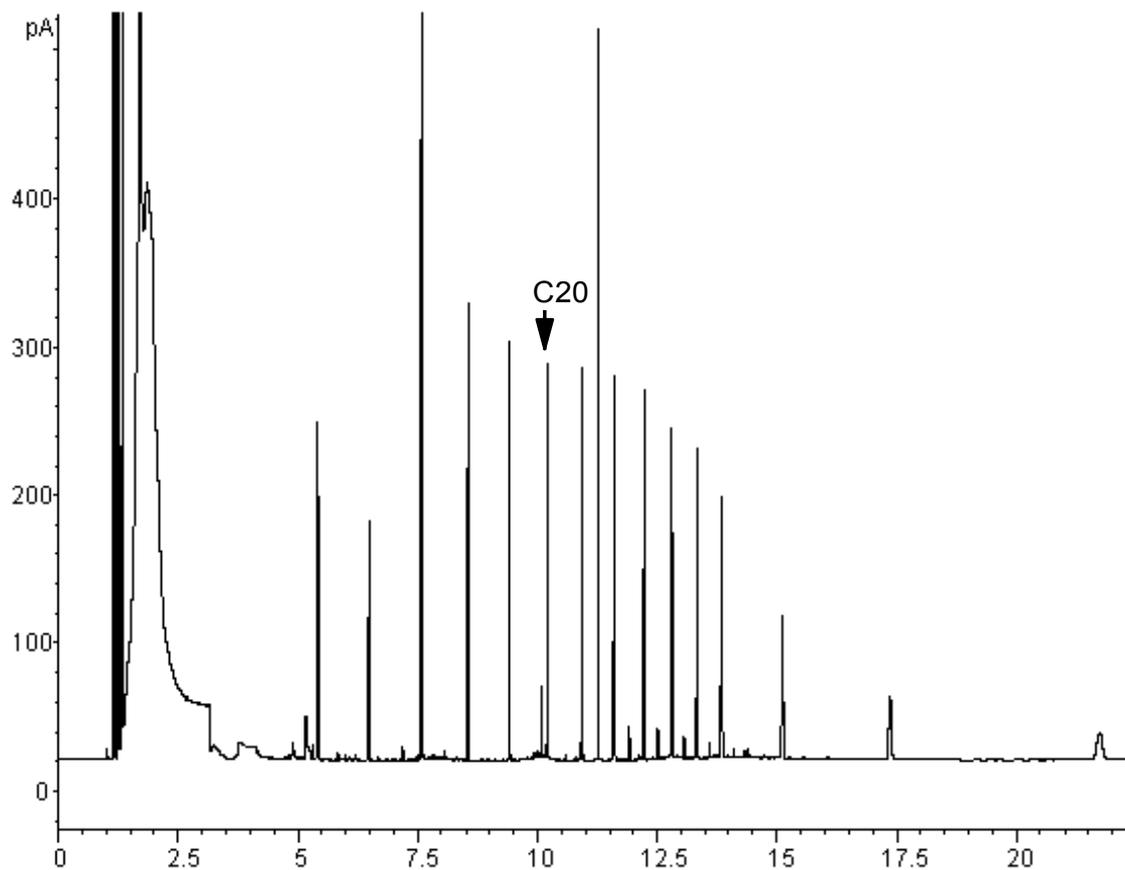
**Figure 13. Chromatogram from one 10  $\mu$ L injection**
