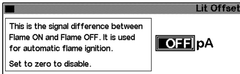
2. Enter a number. The default is 2.0 pA. Enter 0 to disable the automatic reignite function. The setpoint range is 0 to 99.9 pA.
