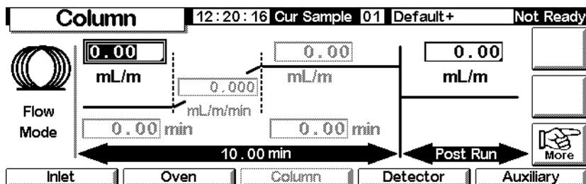
1. The column is in constant flow mode, which is why the ramp setpoints are grayed out. Press **More** and use the Column Mode screen (see [Column modes](#) on page 40) to change to Ramped Flow.
