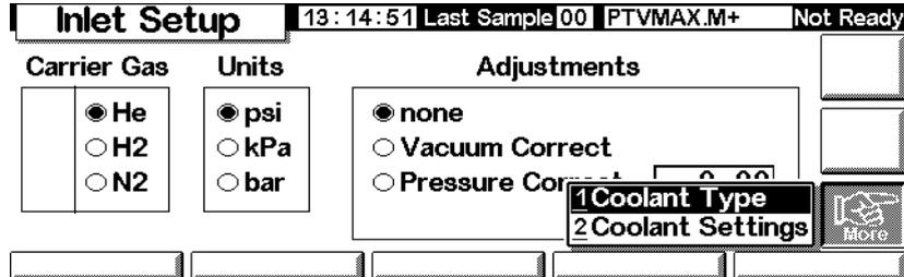
5. Set the type of coolant and press OK. To disable inlet cryo cooling or if no cryo cooling is available, select No Coolant. Press OK.
