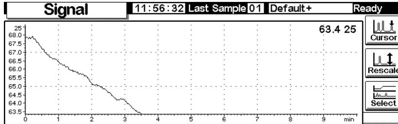
10. To refine the scaling, use ← and → to adjust the horizontal scale and ↑ and ↓ to adjust the vertical scale. In this example, the vertical scale is too sensitive and needs adjusting.
