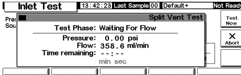
When the GC reaches operating conditions, the test starts automatically. Normally, wait for the test to start. If you want to start the test without waiting for the inlet to reach operating temperature, press **Test Now**.
