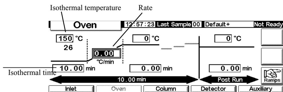
1. Enter the oven temperature for the run in the isothermal temperature field ( $^{\circ}\text{C}$ ). Press **Enter**.
