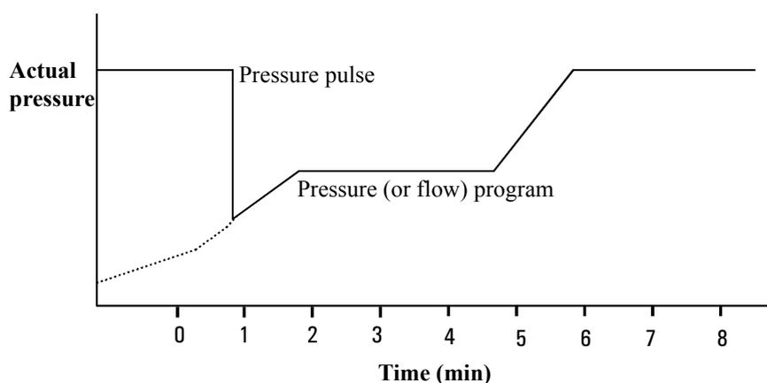
**Figure 3. Pressure pulse and column flow or pressure**
