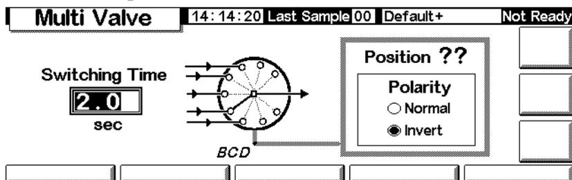
2. Enter a Switching Time in seconds. Viscous samples may require longer times. The default time is 1.0 second.
