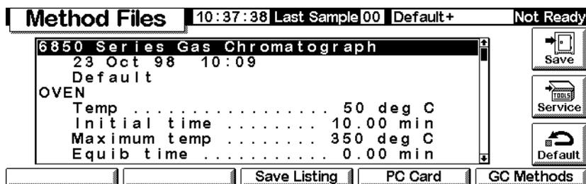
2. The screen displays the beginning of the active method. Use the ↑ and ↓ keys to examine it and verify that all values are correct.
