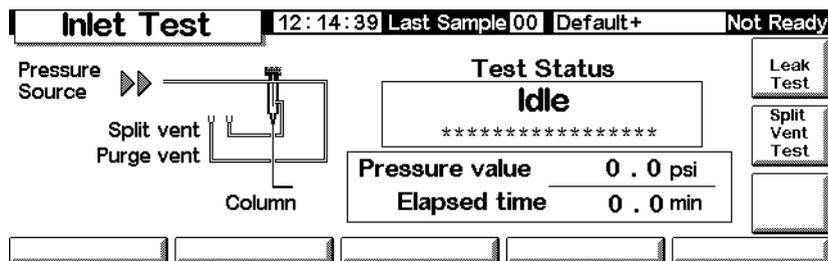
2. Press the Leak Test key.
