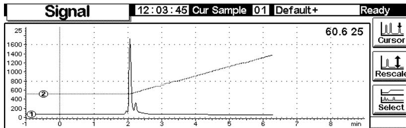
The two plots are superimposed but have independent **Y** scales. Note the small ① and ② that identify the two plots. Use the 1 and 2 keys to select these plots. As you do so, the **Y** scale changes to that of the selected plot.
