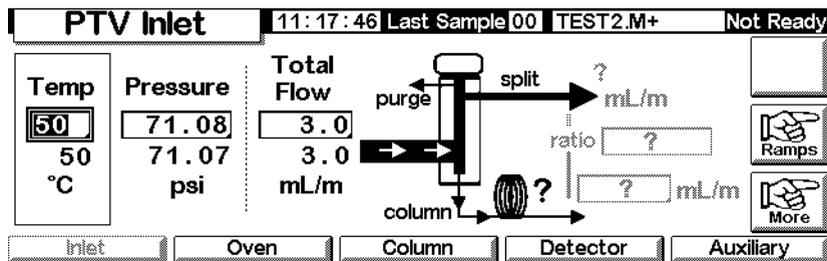
3. Set the inlet temperature and any desired ramps.
