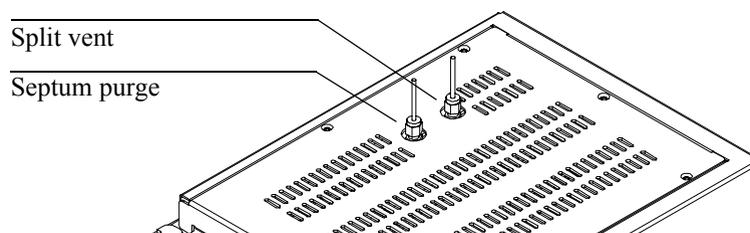
Subtract split vent flow and septum purge flow (see [Table 10](#) for nominal septum purge flows by carrier gas type) from Total flow to get column flow.
