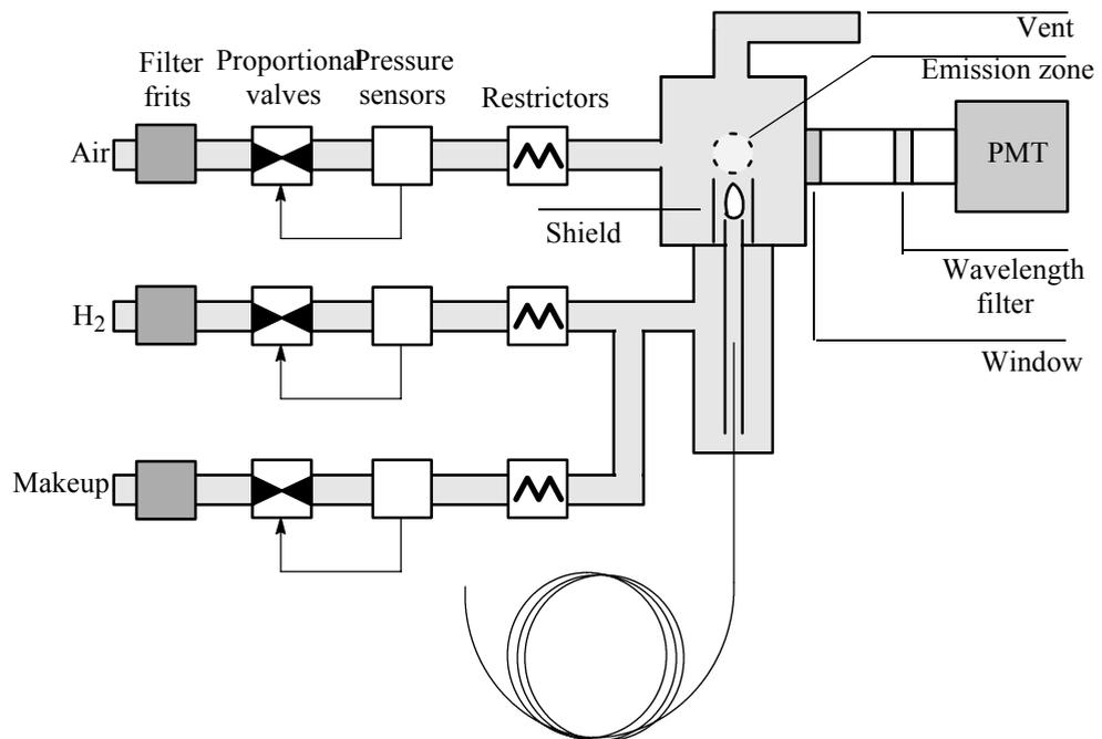
Figure 23. Schematic of a flame photometric detector
