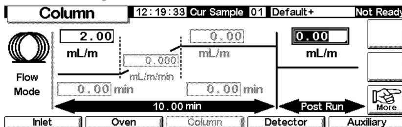
1. Scroll to the psi (pressure mode) or mL/min (flow mode) field.
