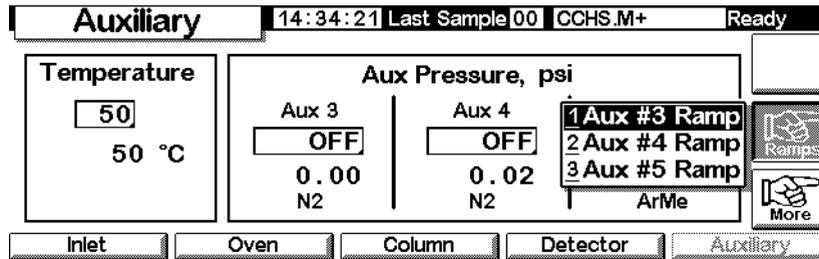
2. Select the ramp you want to set. A pressure ramp table for the selected Aux channel appears. The table for the Aux #3 Ramp is shown below. The others are identical. While this screen lists pressure values in psi units, you specify the units on the Inlet Setup screen.
