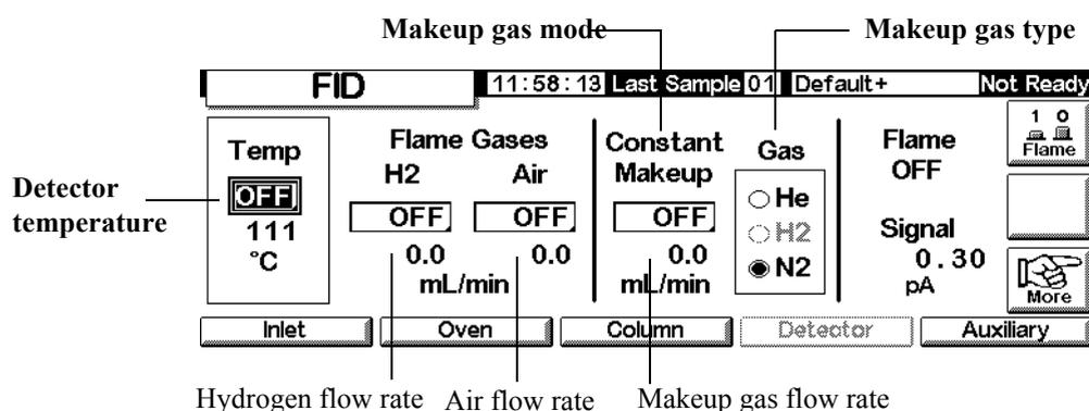
2. Set the detector temperature. The temperature must be greater than 150°C for the flame to light and should be approximately 20°C higher than the highest oven temperature.
