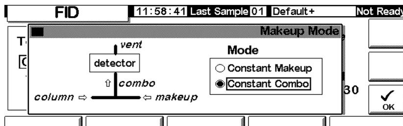
5. Select a makeup mode. Press OK to return to the previous screen. Enter the makeup or combo flow rate.
