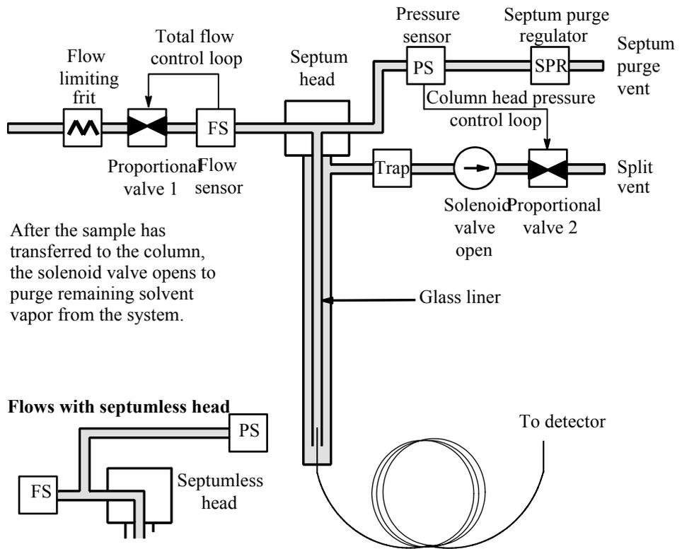
After the sample has transferred to the column, the solenoid valve opens to purge remaining solvent vapor from the system.
