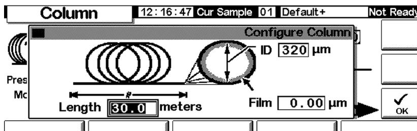
3. Enter values for Length, ID (internal diameter), and Film (thickness).
