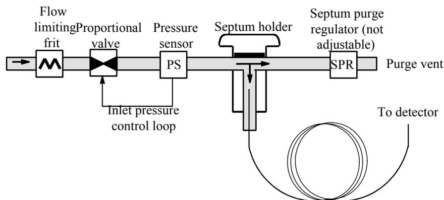
Figure 15. Cool on-column capillary inlet with EPC
