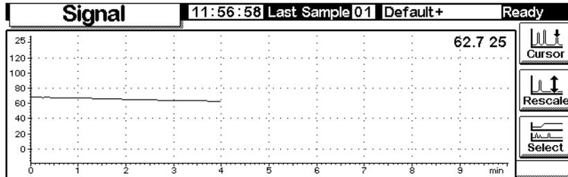
11. Inject a sample—air was used for this example—and press Start. A vertical line marks the start of the run.
