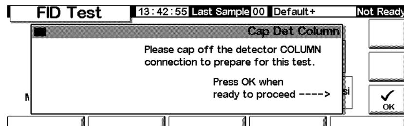
3. After you cap the detector column fitting, the FID Jet Test screen appears:
