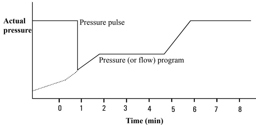
Figure 8. Pressure pulse and column flow or pressure
