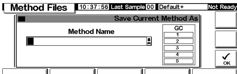
4. The Control Module keys have both labeled and hidden values (see [Table 4](#)). The hidden values apply *only* for entering text in an alphanumeric field, such as the Method Name field on this screen.
