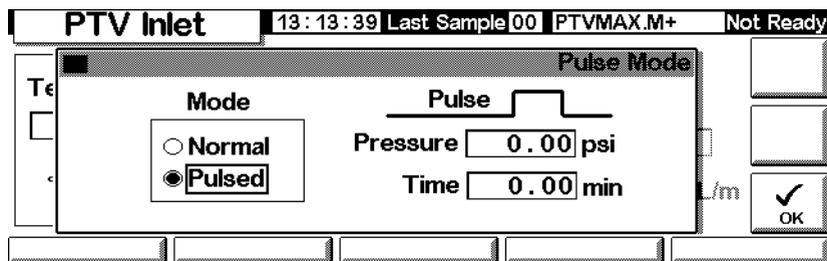
6. Enter values for Pulse pressure and Pulse time and press OK.
