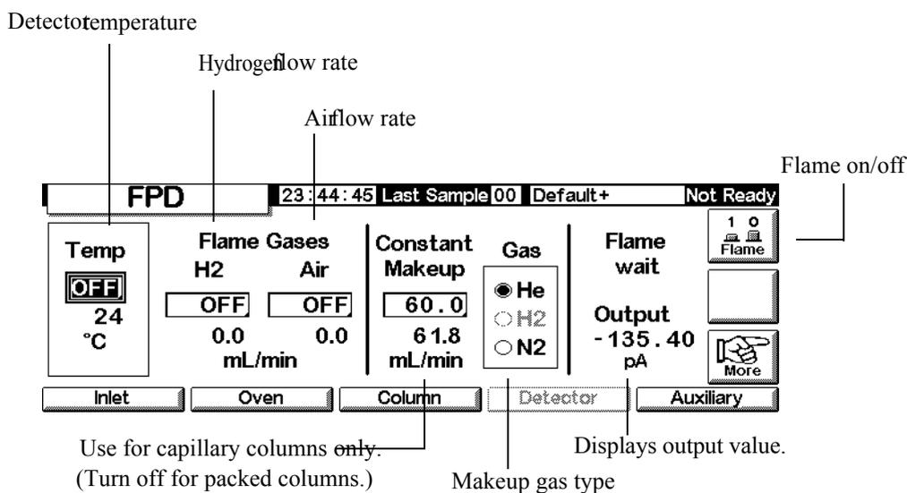
2. Set the detector temperature. The temperature must be greater than 120°C for the flame to light.
