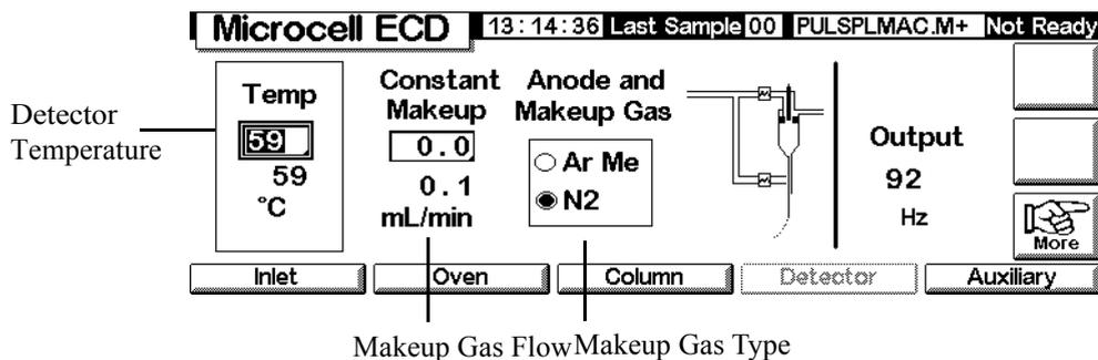
2. Set the detector temperature. To keep the  $\mu$ ECD cell clean, this temperature must be higher than the oven temperature.
