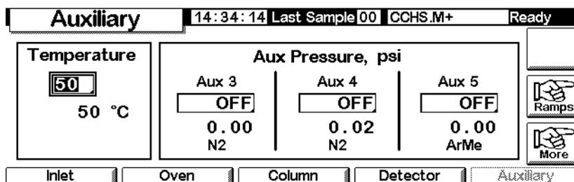
1. Set the temperature and pressures for the appropriate channels.
