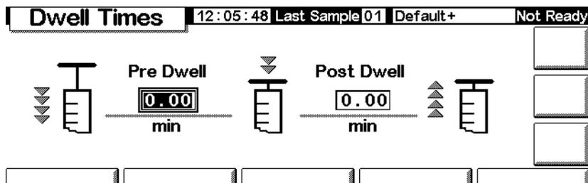
2. Enter your choices. For most uses, both dwell times will be zero. This gives a fast injection with a minimum of boil-out from a hot needle.
