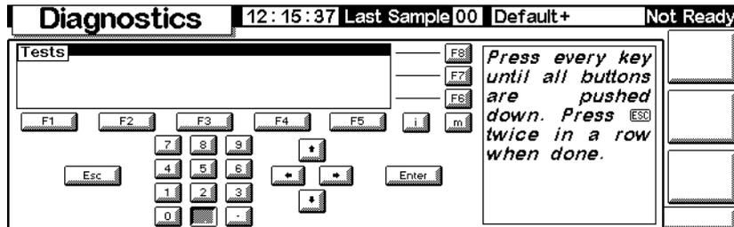
2. Press each key on the Control Module. Its screen image should turn gray.
