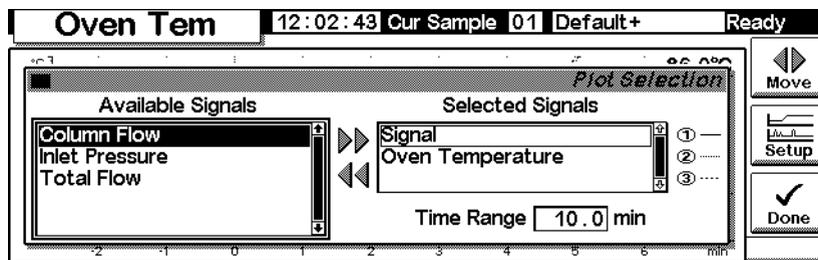
3. Use the  $\uparrow$  and  $\downarrow$  keys, or press 2, to highlight **Oven Temperature**. Press **Setup** to set the **Y Range** for this signal. We suggest a range of 0°C to 150°C.
