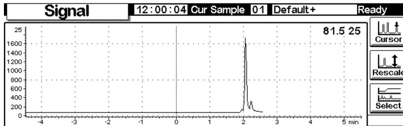
13. To explore the plot in detail, press **Cursor**. An arrow appears on the screen, and the values of time and Signal appear in the top right corner of the screen.
