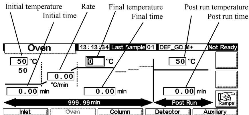
2. Enter the starting conditions—Initial temperature (50°C) and Initial time (2 min).
