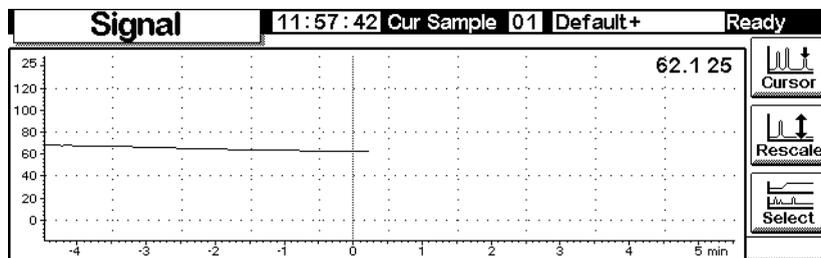
12. When the peak appears, it goes off scale. Wait for the trailing edge to appear, then press **Rescale** to bring the top of the peak on scale. Press  $\downarrow$  once.
