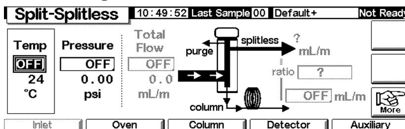
3. If necessary, change the inlet mode to splitless. See [Setting the inlet mode](#) on page 69.
