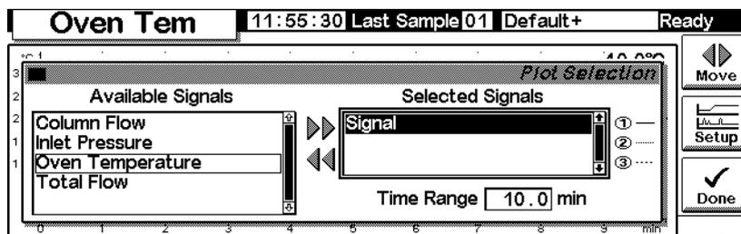
6. Enter a Time Range. This is the width, in minutes, of the plot. If the run lasts longer than this, the plot scrolls off the screen to the left.
