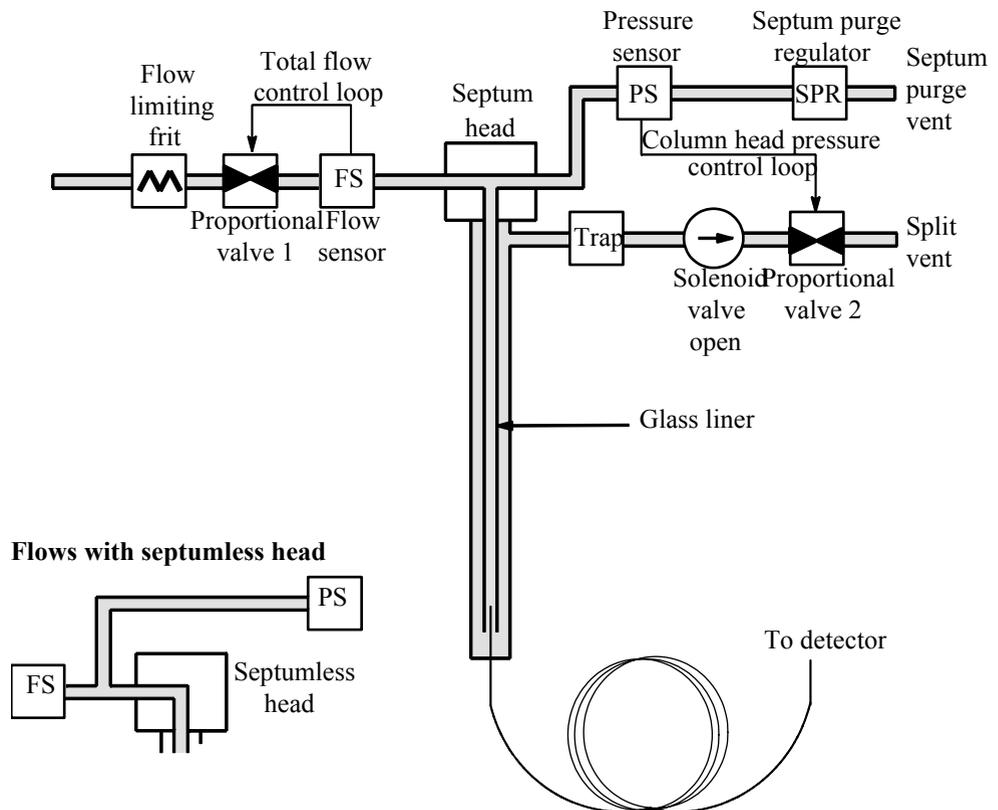
The *total flow* is the sum of the split flow, column flow, and septum purge flow. When you change the total flow, the split ratio and split flow change while the column flow and pressure remain the same.
