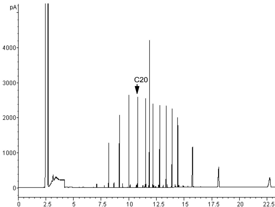
**Figure 14.** Chromatogram from ten 10  $\mu$ L injections
