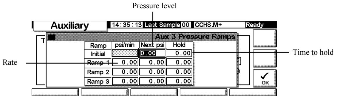
3. Set up to three ramps, entering values for a pressure level, a time to hold that pressure, and the rate at which to move to the next pressure level.
