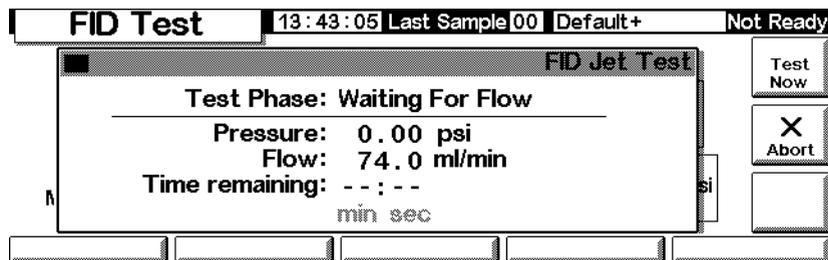
4. When completed, the test result is shown.
