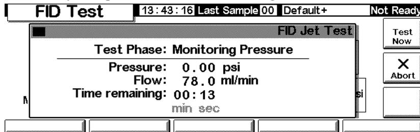
When the GC reaches operating conditions, the test starts automatically. Normally, wait for the test to start. If you want to start the test without waiting for the detector to reach operating conditions, press **Test Now**, then select **Yes** to begin the test immediately.
