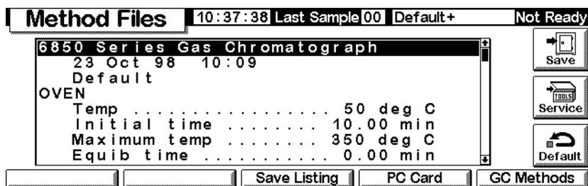
Press **Save Listing**. A text file called *methodname.lst* is saved onto the Method Files screen. Note that the Control Module automatically overwrites any previous version of the listing.
