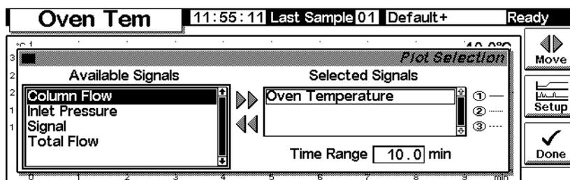
Signal, in the **Available Signals** list, is the signal selected on the detector screen.
