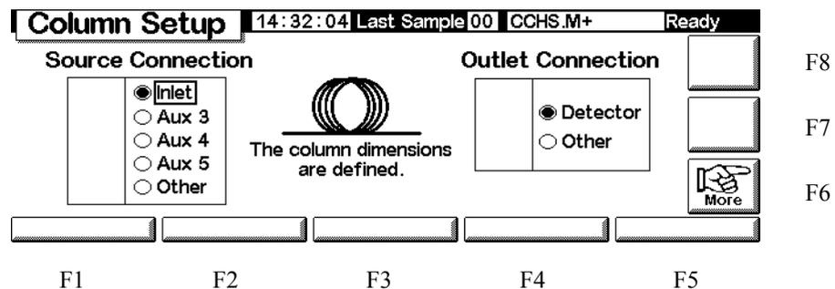
4. Check that the column source and outlet connections are correct. If not, use the ← and → keys to get to the correct set of choices and the ↑ and ↓ keys for the specific choice. Press Enter.
