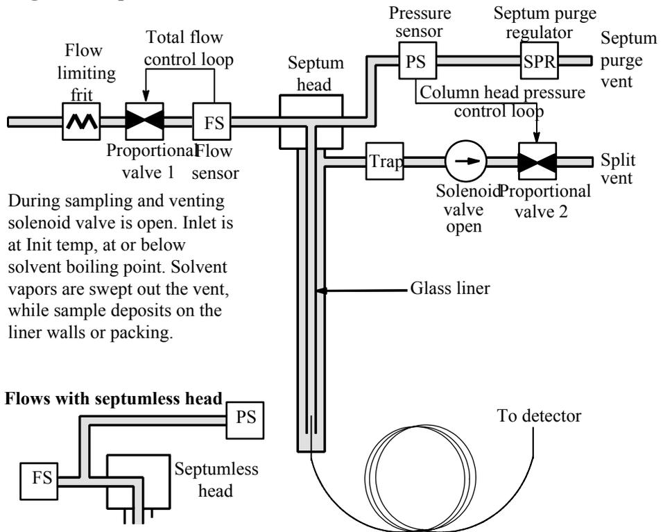
During sampling and venting solenoid valve is open. Inlet is at Init temp, at or below solvent boiling point. Solvent vapors are swept out the vent, while sample deposits on the liner walls or packing.
